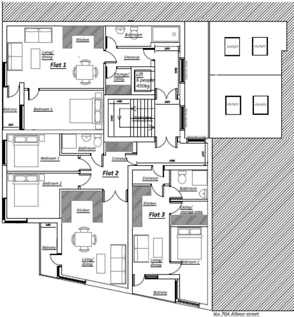
Proposed first, second and third floor layout with one 2 bedroom flat, two 1 bedroom flats, staircase shaft, lift shaft and corridor
